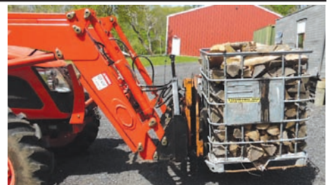
“Rotating forks” let Petrevich lift steel totes loaded with firewood over the side of a dump truck, then rotate them upside down to dump wood directly into truck.
