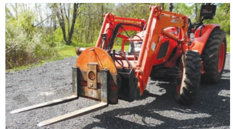
Extending a hydraulic cylinder causes semi-circular steel plate and forks to rotate 180 degrees.
