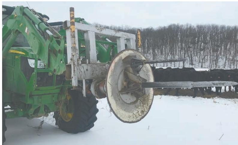
Bale spears are welded to a heavy steel disc and driven by a hydraulic motor that operates off tractor’s hydraulics.
