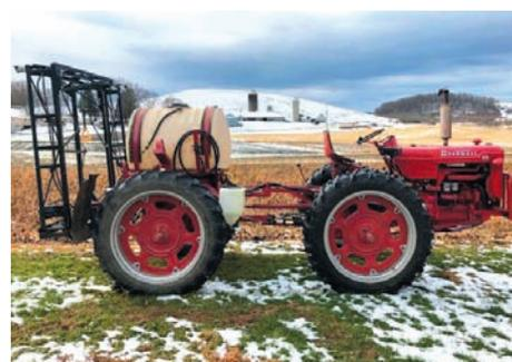
To join the rear ends, Davis built a hinged frame. He then ran a driveshaft from the original pto on the front rear end to the back rear end.
