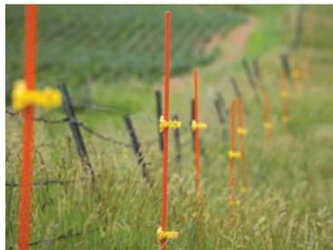
Fully adjustable military grade polymer with UV stabilizer support rings come in 8" 10" & 12" and snap onto 5-ft. steel Herringbone style rib posts that keep rings from rotating once you've locked them in place.
