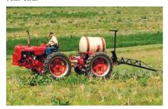
Tractor is powered by a 40 hp. diesel engine out of a junked Ford 3000 tractor. "Works great to spray corn and potato crops," says Davis.
