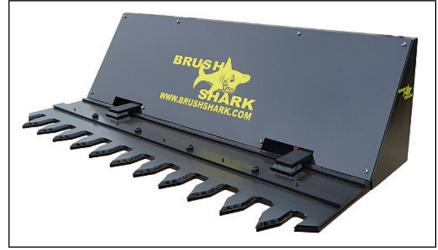
The Brushshark Tree Shear will quickly shear 1/2 to 8-in. diameter trees and brush at ground level. Each cycle takes approximately 1 second and it shears in both directions. Trees and brush up to 3 in. diameter are sheared in one cycle. Material larger than 3 in. diameter, up to 8 in., is efficiently sheared with multiple cycles.
