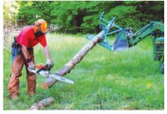
Log picker attaches to loader forks and holds log about waist high, making it easy to cut off pieces.
