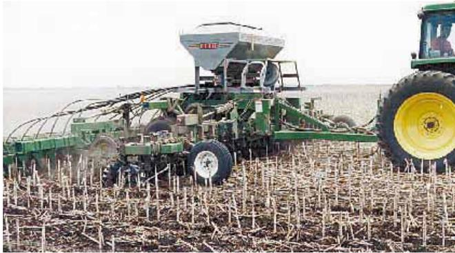
Hiniker air seeder unit mounts on Rawson coulters cart ahead of modified Max-Emerge planter.
