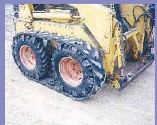
Tracks are made from used rear tractor tires. Steel guides bolt to each side of track at 8-in. intervals.
