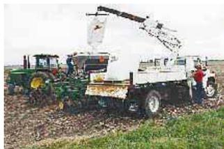
Ellis rented this bulk seed truck with crane from a local seed dealer to load bags into planter's 60-bu. hopper.
