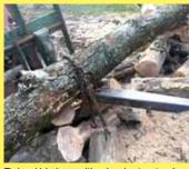
To haul big logs with a loader tractor, I cut off the big end of the log first and then chain the log to a bucket fork. It holds the log tightly in place and I don't have to worry about it rolling off the forks. (Dick Weygandt, Penn.)
