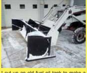
I cut up an old fuel oil tank to make a loader-mounted box blade that I use to remove snow. I cut the tank down the middle and then connected the ends together. Works great any time we don't get a lot of snow at once. If anyone is interested I can provide details on how I made the blade. (John Middaugh, Cooks, Mich.)
