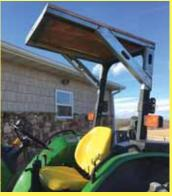
I made this canopy for my 5310 Deere tractor that attaches to the top of the existing rollbar. It's made from heavy metal brackets welded and bolted together, with 1-in. cedar lumber across the top. It's solid enough to last as long as the tractor and provides relief from the sun in the summer. (Larry J. Thompson, St. Mary, Mo. Ph 573 535-0547)
