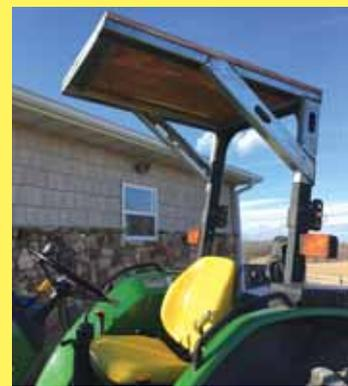
I made this canopy for my 5310 Deere tractor that attaches to the top of the existing rollbar. It's made from heavy metal brackets welded and bolted together, with 1-in. cedar lumber across the top. It's solid enough to last as long as the tractor and provides relief from the sun in the summer. (Larry J. Thompson, St. Mary, Mo. Ph 573 535-0547)
