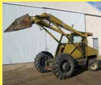
I built this loader tractor almost 60 years ago and still use it regularly. It's built on the chassis of an old Farmer's Union No. 3 tractor. Power is provided by a Dodge slant six engine with an automatic transmission, and the drive axle is a modified planetary axle off a Gleaner C3 combine. The power brakes came off a Chevrolet pickup.
