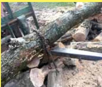
To haul big logs with a loader tractor, I cut off the big end of the log first and then chain the log to a bucket fork. It holds the log tightly in place and I don't have to worry about it rolling off the forks. (Dick Weygandt, Penn.)
