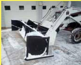
I cut up an old fuel oil tank to make a loader-mounted box blade that I use to remove snow. I cut the tank down the middle and then connected the ends together. Works great any time we don't get a lot of snow at once. If anyone is interested I can provide details on how I made the blade. (John Middaugh, Cooks, Mich.)
