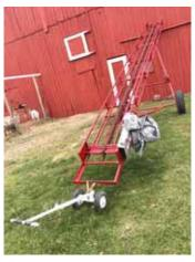
Long-handled, 2-wheeler carrier hooks up to drawbar hitch bolted onto elevator.
