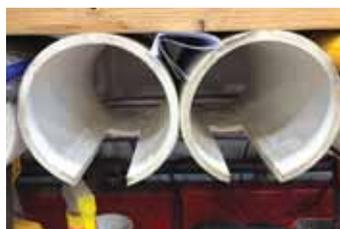
Slots cut into pipes are sized to accommodate different size tool handles.
