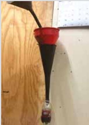
**Tom Chaney, Chrisman, Ill.:** "I didn't like wall-mounted oil funnels dripping oil down my shop wall and making a mess, so I shoved the neck of an empty plastic soda bottle up onto the bottom end of a transmission oil funnel. I place my other funnels inside the top of the transmission oil funnel, so any oil that drips out of them will run down into the bottle. Once the bottle is full I just pull it off and empty it out."
