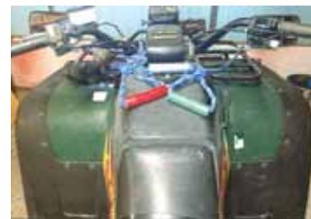
**Center rope extends over 4-wheeler's handlebars and releases the blade lock, allowing blade to rotate.**
