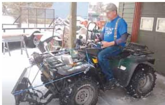
**A homemade system of ropes allows George Collins to quickly change the blade angle on his Arctic Cat 4-wheeler.**
