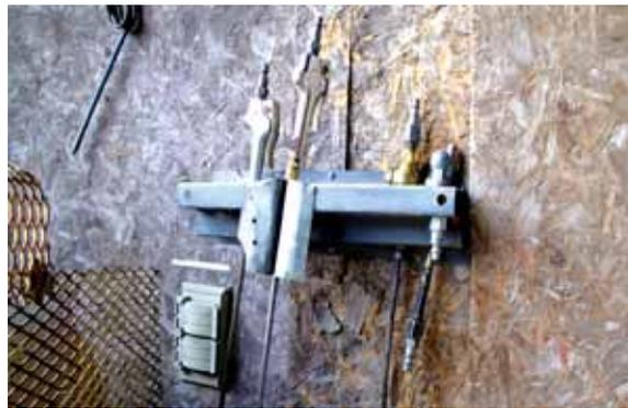
**Lubinski fitted his air blow guns with 1/4-in. steel brake lines and made this wall-mounted rack to store them.**
