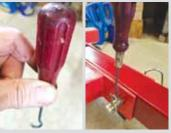
Steve Faber, Tiffin, Ohio: "Hitch pins are sometimes hard to pull so I made a hitch pin puller using an old screwdriver handle. I removed the screwdriver shank and drilled a hole all the way through the handle. Then I drove a heavy #9 wire into the handle and bent a hook into one end. I flattened the other end so it can't pull out of the handle. I keep one of these in my tractor toolbox and one in my shop. Very handy."
