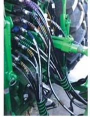
Outback Wrap hydraulic hose markers come in different colors, and are coilshaped to wrap around the hose and grip the surface.
