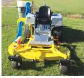
All-hydraulic mower is powered by a Chevy Geo 3-cyl. gas engine that belt-drives hydraulic pumps.
