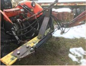
mounts on tractor 3-pt. and uses an attached hydraulic cylinder to move rake back and forth.
