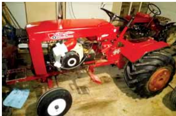
Luke Yoder repowered this WheelHorse gas garden tractor with a Yanmar 6 1/2 hp. diesel engine. “I like how it sounds and how it blows out the smoke,” he says.
