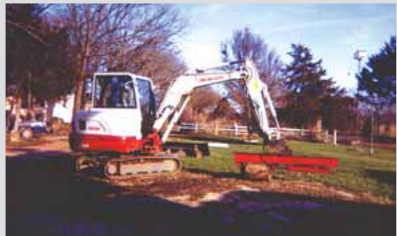
Log splitter mounts in place of the bucket on Zimmerman's Takeuchi compact excavator.
