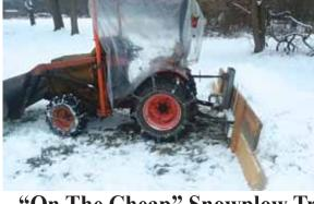
"Poor man's" snowplow tractor is fitted with a homebuilt, 10-ft. wooden snow blade and a "shower curtain" cab.
