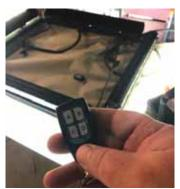
Remote-controlled fob can be used to operate the lights individually or all at the same time.
