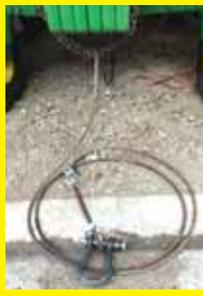
I run a steel cable from the clevis up to the tractor's front weights and wrap it around them until it's needed. If the tractor gets stuck, I just unwrap the cable and attach it to the pulling tractor. A short chain wrapped around the weight box keeps the cable running straight ahead.
