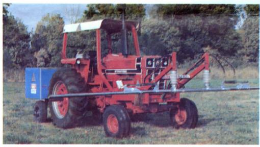
Entire length of the horizontal bar is energized with electricity to "zap" taller-growing weeds on contact.
