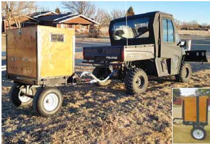
Flexible pipe delivers exhaust from towing vehicle back to a manifold that warms up compartment under cart's floor.
