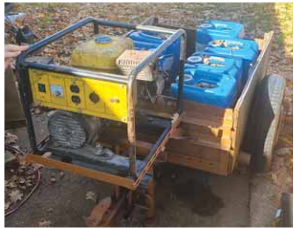
Cart-mounted generator is used to operate a 110-volt sump pump that supplies water for Snyder's garden.
