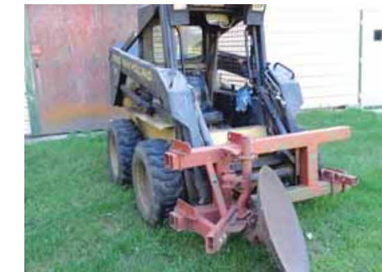
Big 31-in. dia. "blade" weighs 200 lbs. and can cut through sod up to 6 in. deep. Worked great to dig a trench to drain water away from a house.
