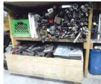
Cut-off square tubing is stacked on shelf under workbench, with smaller pieces of tubing slid inside them.
