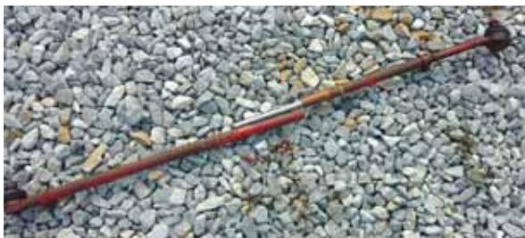
Spencer used part of the steering rod on an older Ford 8N to replace the bad back joints on his 1951 model.
