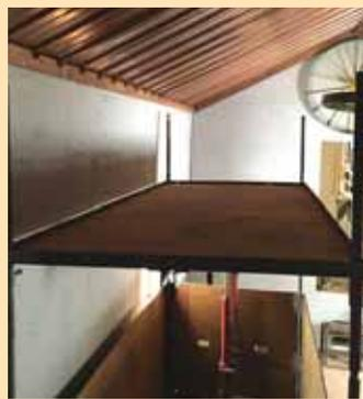
Scaffold has a fixed set of 4 vertical support pipes and a 4 by 8-ft. platform that can be raised up to 9 ft. high.
