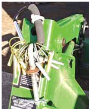
Johnson stores hitch and lynch pins on a 5-in. aluminum carabiner that's secured by an eye bolt installed on his tractor's loader post.
