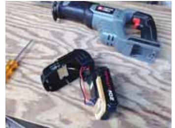
Kent MacDougal came up with an adapter that lets him use a 20-volt Porter Cable battery on an 18-volt Porter Cable tool.
