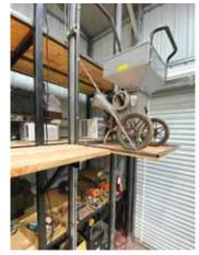
Gradek built this shop elevator to access an upper storage area in his shed. It raises and lowers a wooden platform that rides up or down a pair of tracks.
