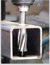
Blair Equipment Co., Swartz Creek, Mich. ph 800 426-7818; www.@ blairequipment.com: Their extended reach metal hole cutters provide up to 2 1/2 in. of additional reach. They allow you to drill holes in pipe, tubing and plate materials up to 1/4 in. thick. The company says they're ideal for making single pass holes in hollow tubing because you can drill 2 perfectly lined up holes. They can be used in 3/8 or 1/2-in. hand drills or drill presses. Available individually or in a kit.
