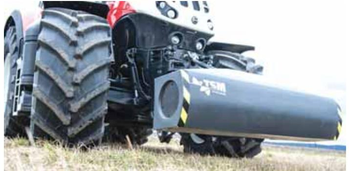
Top Soil Mapper identifies soil compaction depth on-the-go and tells you how deep to rip. It can be used with an automatic tillage control kit that installs on your cultivator or subsoiler.
