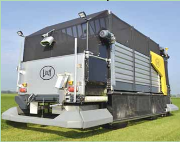
Lely's prototype “hay robot” is designed to harvest fresh grass and store it in a holding tank, then haul it to the barn and feed it to cattle.
