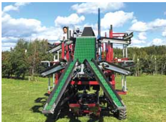
Robotic apple harvester comes with a computer-vision sorting system that matches the picking speed of 6 workers. Two workers pick at ground level, and 4 from platforms on harvester's sides.
