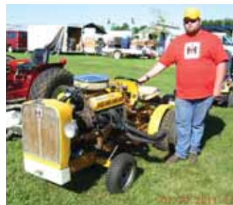
Matt Brand replaced the original 1-cyl., 7 hp. engine on his 1961 Cub Cadet with a V-8 carbureted engine out of an old Jeep. "I built it mainly as a conversation piece," he says.
