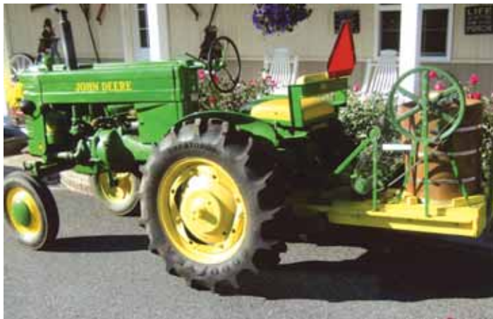
Ice cream maker is belt-driven by the gearbox off an old bin sweep auger, which is attached to tractor pto.
