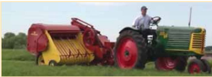
Lano is shown driving his Oliver 66 and pulling a New Holland 77 baler, the first model the company built with a right side pickup and steel teeth instead of an apron.
