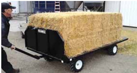
Kramble makes several versions of electric work carts, including this 4 by 8-ft. barn cart. A 12-volt rear-drive motor provides variable speed forward and reverse.
