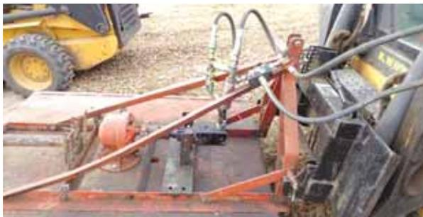
Vogelzang removed mower's pto shaft and installed a hydraulic motor to match the hydraulic output of his skid loader.
