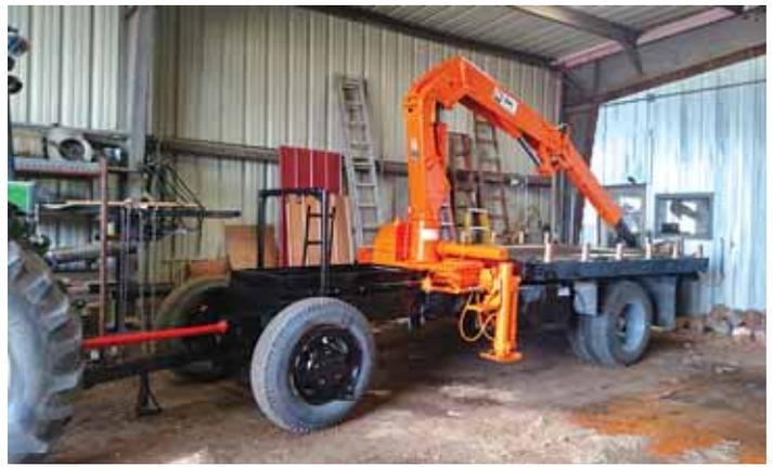
**To convert boom truck to a trailer Cerveny cut down the truck’s frame, added a tongue on front, and reversed the front axle. He also extended linkage to truck’s driveline so he could power the boom with a tractor pto.**
