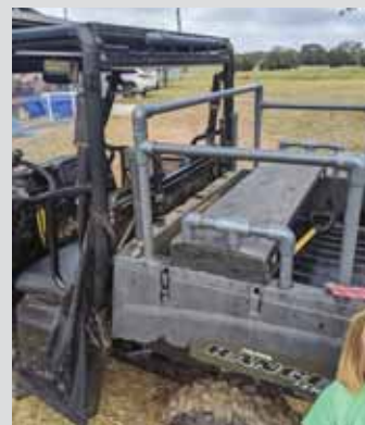
Home-built wooden bench in Ranger bed converts to a headache rack (above). Painted wooden roof on top of cab is strong enough to stand on and reach high places.
