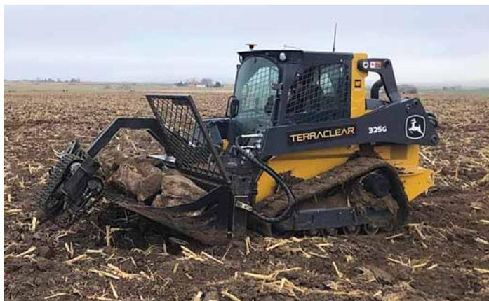
**Robotic rock picker uses a drone to make field maps of pick-worthy rocks in your field. A loader-mounted picker, equipped with twin rubber tracks on an articulating arm, sees and picks the rocks and spits them back into bucket.**
