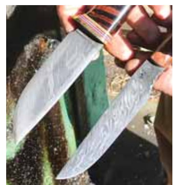
Godlesky selectively uses bandsaw mill blades to make high quality Damascus steel knives.
