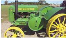
Deere D tractors built after 1926 featured the side-mounted upward exhaust first designed by Sands.
