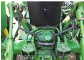
Anti-sway assembly (right) holds lift arms securely in place for easier and safer equipment hookup. Locking bar installs on lift arms to hold them up when not in use.
