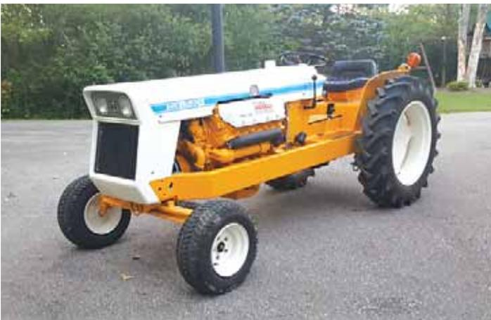
Repowered Cub Cadet Lo-Boy was lengthened by 22 in. to make room for a 500-hp., 7.3-liter Power Stroke diesel engine off a Ford F-350 pickup.
