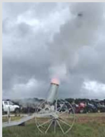
Jim Esbenshade built this cannon out of an oxygen cylinder, mounting it on an axle fitted with steel wheels. "We can make it shoot a bowling ball 2 miles," he says.
