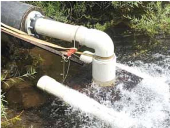
PVC float system is made from 2 parts - a 90-degree elbow with a 6 by 8-in. bushing on the bottom, and an H-shaped float with a 6-in., center-mounted vertical cap.
