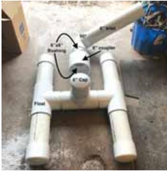
As float rises with the water level, the vertical cap puts pressure on bushing to seal off a pond inlet pipe.
