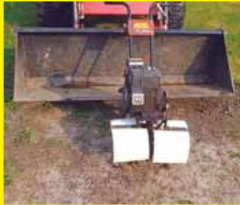
I wanted to go through my corn rows with a small rototiller without getting wrapped up in the leaves. So I cut a piece of 12-in. dia. pvc in half and made some quick-mount brackets so I can put them on when needed. Worked great. I also use them around caged tomatoes and other garden plants as well. **(Jim Lacey, Dell Rapids, S.Dak.)**
