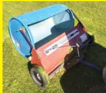
I found a 38-in. pull-type lawn sweeper at the local salvage yard. The owner threw it away after the canvas bag on it rotted away due to long term outdoor storage. I thought about building a tin or plywood hopper to replace the bag, but then I saw a nearby 55-gal. drum that was nearly as tall as the sweeper was wide. Being a plastic food grade drum, it was light and easy to work with.
