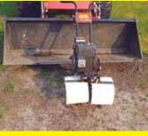
I wanted to go through my corn rows with a small rototiller without getting wrapped up in the leaves. So I cut a piece of 12-in. dia. pvc in half and made some quick-mount brackets so I can put them on when needed. Worked great. I also use them around caged tomatoes and other garden plants as well. (Jim Lacey, Dell Rapids, S.Dak.)
