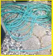
I've found that to keep hoses from tangling, it's best to lay them in a figure eight instead of a circle. It also keeps the twist out of the hose since each half wrap reverses direction.
