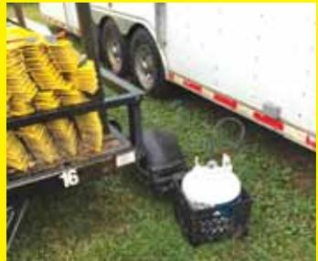
Milk crates work great to hold propane tanks in the back of pickups or on trailers. Keeps them from rolling around. **(Gary Swensen, Yankton, S.Dak.)**
