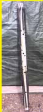
Here's how I store bungee straps. Drill holes in a piece of pvc pipe and hook the straps over the end and into whatever hole matches the length. Eliminates having a pile of straps and you can see at a glance which strap is the one you need. **(Cal Miner, Willmar, Minn.)**
