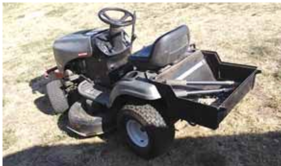
Dennis Gingrich used the lid off an old Weber barbecue grill to make a handy utility box for his riding mower.
