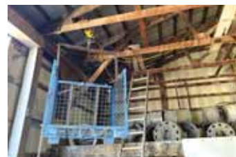
Metal lift box is raised and lowered by an electric winch and operated by a handheld control.
