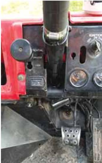
**Kokur replaced the factory steering column assembly on his Kawasaki Mule with one off a Toyota Prius. He also attached the Toyota's steering computer module under the dash and wired it to the battery.**
