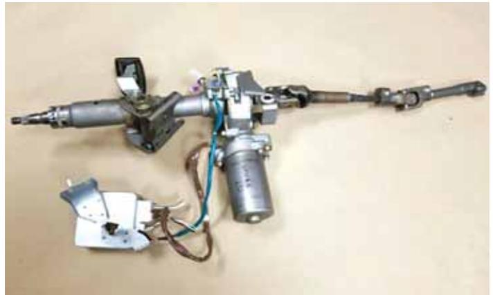
**He cut the Toyota power and car control harness to make pigtail connections for the steering module.**
