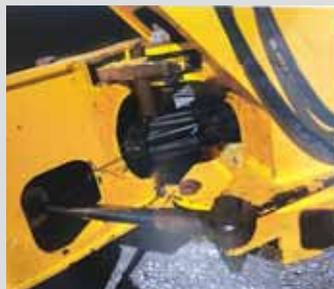
**Marvin Martin, Elkton, Ky.:** “On a Wrangler 4500 loader the hoses wanted to rub as they went through the frame at the articulation joint. I double wrapped the hoses with a piece of ratchet strap and secured them with zip ties temporarily. I then wrapped wire around the ratchet strap and tied it off, securing to the frame on one side. I used medium tension on the wires. I had to remove the front side access cover to reach the hoses.”
