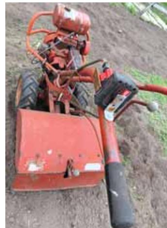
The coil on Podoll’s rototiller was shot, but he got the machine going again by installing a 12-volt coil with bracket (below) and wiring it to a cordless tool battery strapped onto the handlebar.
