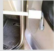
"My pickup has manual crank windows, and when I'm behind the steering wheel I can't reach all the way over to open the passenger window. I attached a short piece of pvc pipe over the handle, so I can insert a broom handle inside the pipe that lets me crank the window up or down. I use my left hand to hold the broomstick handle steady and my right hand to rotate the handle. Works great."
