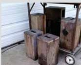
"I used 2-in. boards to build several boxes that serve as portable workbenches. Handhold slots cut into the tops of the boxes make them easy to move around. When I'm working on a bigger project, I might use 3 or 4 boxes at the same time to hold material in place.
