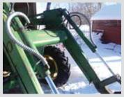
Duane Kuesel, Elmwood, Wis.: "I prolong the life of the hydraulic lines on my front-end loader by slipping steel electrical conduit over them. It saves the rubber from being peeled off when pushing brush and tree branches. Plastic conduit could also be used."
