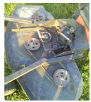
Aaron Miller built a bigger 48-in. mower deck for his DR brush mower, using the pulleys and components from an old Deere mower.
