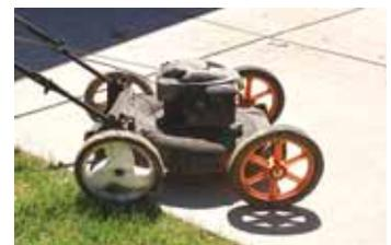
Mower's 4 large wheels provide enough extra clearance to cut down brush.
