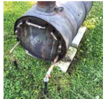
Studer installed 12 copper tubes inside barrel stove. Tubes gather heat off stove, and swimming pool's pump circulates the heated water through underground tubes into pool.
