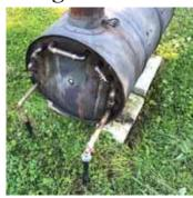
Studer installed 12 copper tubes inside barrel stove. Tubes gather heat off stove, and swimming pool's pump circulates the heated water through underground tubes into pool.
