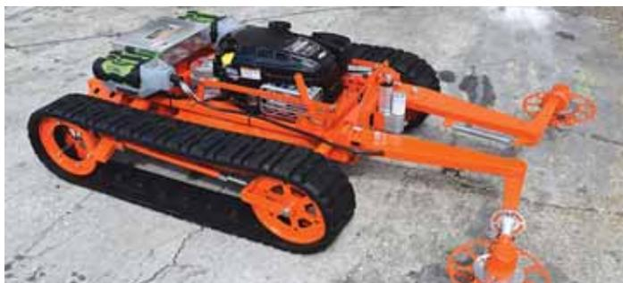
Goat robotic 22T solar lawn mower is designed to mow under solar panel arrays. It's just 18 1/2 in. tall and comes with 2 trimmer arm attachments.
