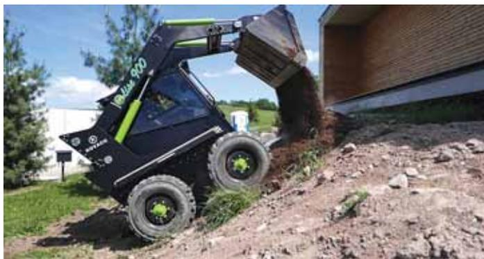
More than 40 different attachments are available for the Elise 900 electric skid loader. It can be operated remotely using a mobile phone for display and control.
