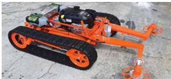
Goat robotic 22T solar lawn mower is designed to mow under solar panel arrays. It's just  $18\ 1/2$  in. tall and comes with 2 trimmer arm attachments.
